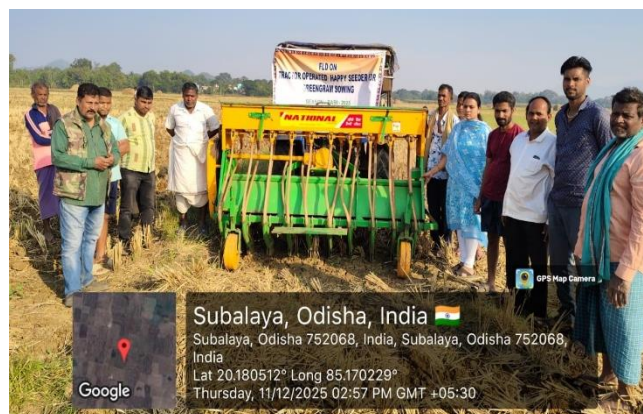
Demonstration on Tractor Operated Happy Seed drill for Greengram sowing
